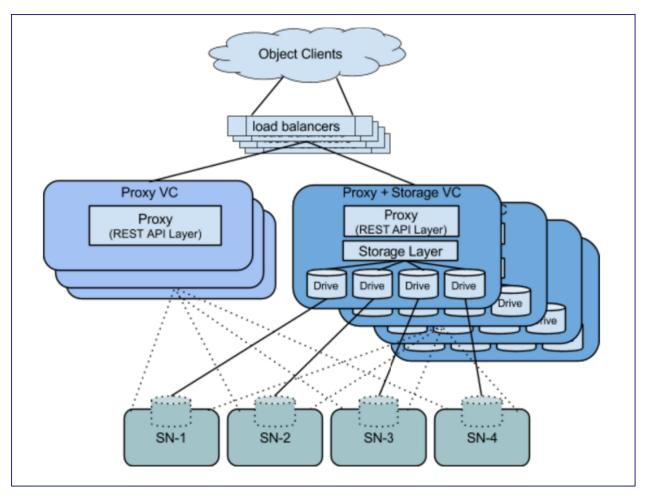
This figure shows high level logical view of VPSA Object Storage. It is a Virtual Object Store cluster, with two distinct layers:
